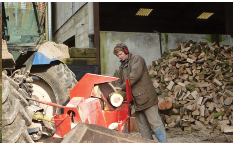
Most hedge material is processed with a saw bench. Ross Dickinson, 2017
