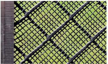
Close-up of a heavyweight, reinforced double-mesh tree guard ( $25 \times 25 \text{ mm}/ 2.5 \times 2.5 \text{ mm}$ ). This is suitable for agroforestry
